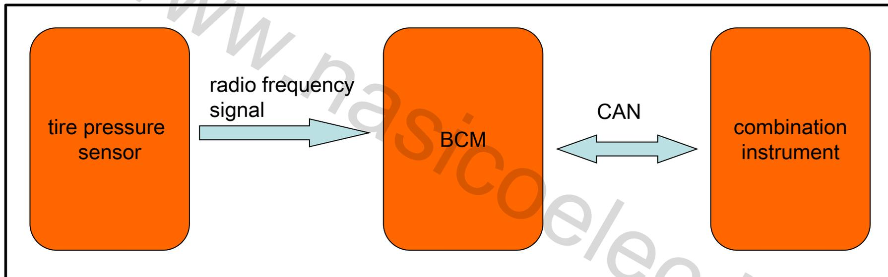
Remark: The wireless communication frequency of tire pressure sensor and car body controller is 433MHz.
