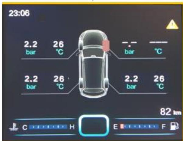
When the speed  $> 30\text{km/h}$ , if the TPMS does not receive one or more radio frequency signal after 10 min, then TPMS will do system breakdown alarm. The instrument will display “Please check TPMS.” At the same time, indicating sign will flicker for 75s and then be normally on.
