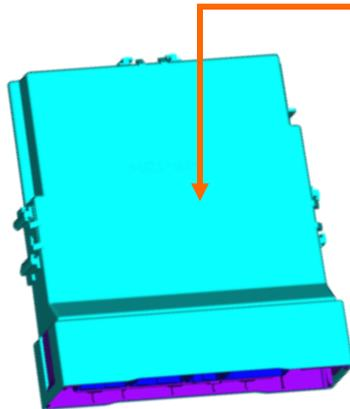
➤ PEPS control module is installed under the FR A pole, which is the main control module of PEPS system.
