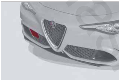
Front Bumper Radar Location
