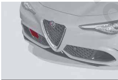
Front Bumper Radar Location
