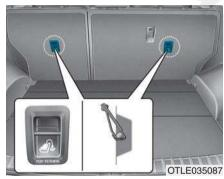
Top-tether anchorages for Child Restraint Systems are located on the rear of the seatbacks.
