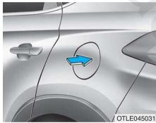
1. To open the fuel filler door, press the center edge of the fuel filler door.
