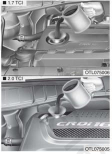
Use only the specified engine oil. (Refer to "Recommended lubricants and capacities" in chapter 8.)
