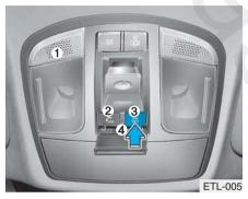
Elements of the system ERA-GLONASS, installed in passenger compartment:
