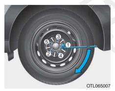
13. Use the wheel lug nut wrench to tighten the lug nuts in the order shown. Double-check each lug nut until they are tight. After changing tires, we recommend that an authorized HYUNDAI dealer tighten the lug nuts to their proper torque as soon as possible. The wheel lug nut should be tightened to 9~11 kgf·m (65~79 lbf·ft).
