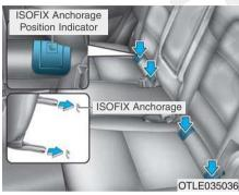
ISOFIX anchorages are located between the seatback and the seat cushion of the rear seat left and right outboard seating positions, indicated by the symbols  $\mathbf{k}_{i}$ .
