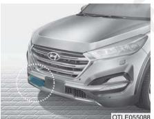
The sensor is to maintain a certain distance from the vehicle in front. However, the smudged sensor lens with foreign substances, such as snow and rain, adversely affects the sensing performance. It may even temporarily cancel the AEB. Always keep the sensor lens clean.
