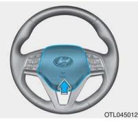
To sound the horn, press the area indicated by the horn symbol on your steering wheel (see illustration). The horn will operate only when this area is pressed.
