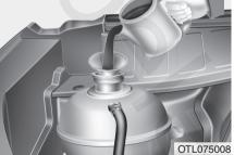
Check the condition and connections of all cooling system hoses and heater hoses. Replace any swollen or deteriorated hoses. The coolant level should be filled between MAX and MIN marks on the side of the coolant reservoir when the engine is cool.
