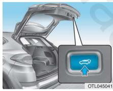
• Press the power tailgate inner switch for approximately one second when the tailgate is opened.
