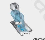
tions. + (Up) : Push the lever forward once to shift up one gear.
