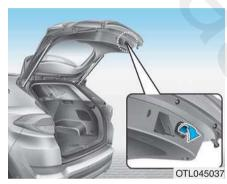
Lower and push down the tailgate firmly. Make sure that the tailgate is securely latched.
