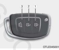
To lock the doors, press the Door Lock button (1) on the remote key.
