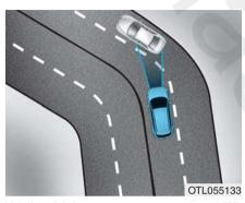
While driving on a curve, the AEB may recognize the vehicle in front in the next lane. Pay great caution, and, if necessary, depress the brake pedal.
