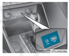
You can use an AUX port to connect audio devices and an USB port to plug in an USB and also in an iPod<sup>®</sup> port.
