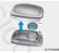
If the Smart Key is not working properly, try replacing the battery with a new one.
