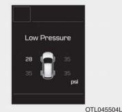
This warning message illuminates if the tire pressure is low with the ignitions switch in ON position.
