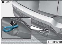
If towing is necessary, we recommend you have it done by an authorized HYUNDAI dealer or a commercial tow truck service. If towing service is not available in an emergency, your vehicle may be temporarily towed using a cable or chain secured to the emergency towing hook at the front (or rear) of the vehicle.
