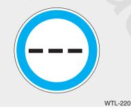
• The symbol is displayed on the instrument cluster and the navigation, when the SLIF does not detect any reliable speed limit information.
