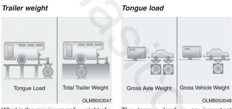
What is the maximum safe weight of a trailer? It should never weigh more than the maximum trailer weight with trailer brakes. But even that can be too heavy. It depends on how you plan to use your trailer. For example, speed, altitude, road grades, outside temperature and how often your vehicle is used to pull a trailer are all important. The ideal trailer weight can also depend on any special equipment that you have on your vehicle.
