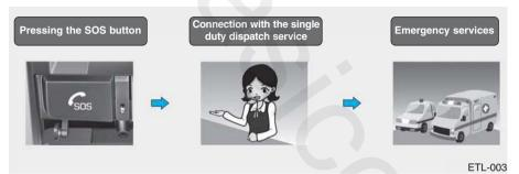
Driver or passenger manually can make an emergency call in the single duty dispatch service, by pressing SOS button to call the necessary emergency services.
