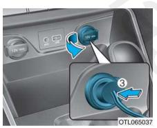
7. Connect between compressor and the vehicle power outlet using the cable and connectors.
