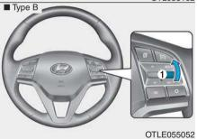
Push the lever (1) up (RES+) and hold it, while monitoring the SET speed on the instrument cluster. Release the lever when the desired speed is shown and the vehicle will accelerate to that speed.
