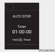
This mode displays the elapsed time of Auto stop by "Idle stop and go system".
