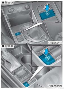
The Downhill Brake Control (DBC) supports the driver come down a steep hill without depressing the brake pedal.
