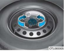
Turn the winged hold down bolt counterclockwise to remove the
