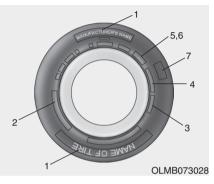
This information identifies and describes the fundamental characteristics of the tire and also provides the tire identification number (TIN) for safety standard certification. The TIN can be used to identify the tire in case of a recall.
