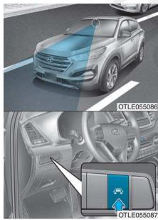
The Lane Keeping Assist System detects lane lines on the road, and assists the driver's steering to help keep the vehicle between lanes. When the system detects the vehicle straying from its lane, it alerts the driver with a visual and audible warning, while applying a slight countersteering torque, trying to prevent the vehicle from moving out of its lane.
