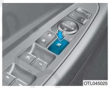
The driver can disable the power window switches on the rear passengers' doors by pressing the power window lock switch. When the power window lock switch is pressed:
