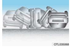
Front air bags may not inflate in rollover accidents because front air bag deployment would not provide additional occupant protection.
