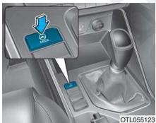
The flex steering wheel controls the steering effort in accordance with the driver's preference and road conditions.
