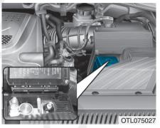
If an electrical system does not operate with no blown fuse in the engine room and inner fuse box, the main fuse inside the battery (+) cap may be blown.
