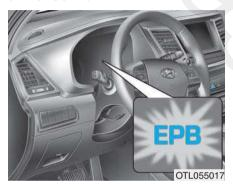
If the EPB malfunction indicator remains on, comes on while driving, or does not come on when the Engine Start/Stop button is changed to the ON position, this indicates that the EPB may have malfunctioned.
