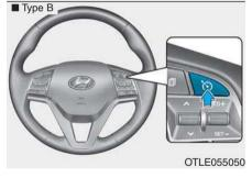
1. Press the CRUISE / (\*) button on the steering wheel to turn the system on. The CRUISE indicator will illuminate.
