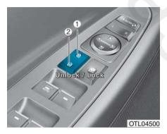
When pressing the  $(\boxdot)$  portion (1) of the switch, all vehicle doors will lock.
