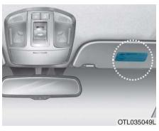
Air bag warning labels are attached to alert the passengers of potential risks of the air bag system.
