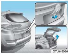
• Once the tailgate is opened and then closed, the tailgate locks automatically. (All doors must be locked.)
