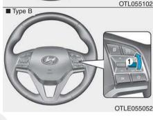
Push the lever (1) up (RES+). If the vehicle speed is over 30 km/h (20 mph), the vehicle will resume the preset speed.
