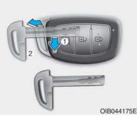
Press and hold the release button (1) and remove the mechanical key (2). Insert the mechanical key into the key hole on the door.
