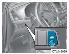
• Press the power tailgate button for approximately one second when the tailgate is opened.
