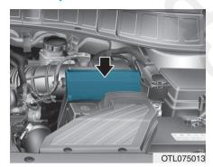
The air cleaner filter can be cleaned for inspection using compressed air.
