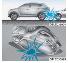
• The vehicle is involved in a side/rear collision or a rollover. The active hood lift system activates only in a frontal collision.
