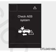
This warning message illuminates if there is a malfunction with the Autonomous Emergency Braking (AEB) system. We recommend that the vehicle be inspected by an authorized HYUNDAI dealer.
