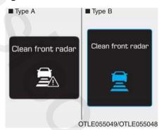
When the sensor cover or the sensor lens is smudged with the foreign substances, such as snow or rain, the AEB operation may temporarily stop. In this case, the warning message appears to warn the driver. This is not a malfunction with the AEB. To operate the AEB again, remove the foreign substances.
