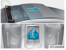
If you pull the sunroof control lever backward to the second detent, the sunshade will slide all the way open then the sunroof glass will slide all the way open. To stop the sunroof movement at any point, pull or push the sunroof control lever momentarily.
