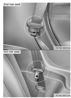
Routing the seat belt webbing through the rear seat belt guides will help keep the belts from being trapped behind or under the seats.
