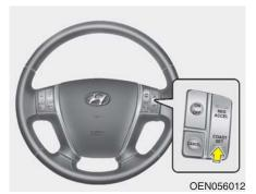
Push the COAST/SET switch, and release it at the desired speed. The SET indicator light in the instrument cluster will illuminate. Release the accelerator at the same time. The desired speed will automatically be maintained.
