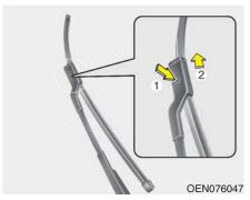
4. Press the button and slide the blade assembly upward.
