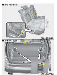
4. Pull on the seatback folding lever, then fold the seat toward the front of the vehicle. When you return the seatback to its upright position, always be sure it has locked into position by pushing on the top of the seatback.
