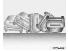
Air bags may not inflate in rollover accidents because air bag deployment would not provide protection to the occupants.
