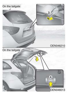
The power tailgate can be opened and closed automatically with the transmitter (or smart key), the main control button on the driver side crash pad, or the sub control button or handle switch on the tailgate.
