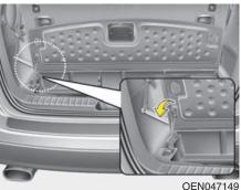
2. Pull out the support rod and hold the cover open with the support rod by inserting the free end of the rod into the slot on the side of the box.
