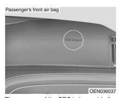
The purpose of the SRS is to provide the vehicle's driver and/or the front passenger with additional protection than that offered by the seat belt system alone in case of a frontal impact of sufficient severity. The SRS uses sensors to gather information about the driver's seat position, the driver's and front passenger's seat belt usage and impact severity.
