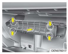
Remove the climate control air filter case pulling out both sides of the cover.
