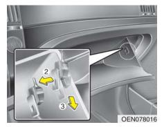
With the glove box open, remove the stoppers on both sides to allow the glove box to hang freely on the hinges.
