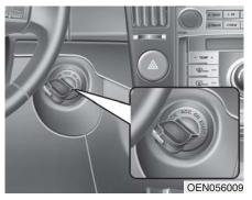
If the battery is weak or the smart key does not work correctly, you can start the engine by inserting the smart key in the ignition switch.
