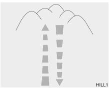
When you are driving up or down hills drive as close to straight up and down the hill as possible. Use extreme caution in going up or down steep hills, since you may flip your vehicle over depending on the grade, terrain and water/mud conditions.
