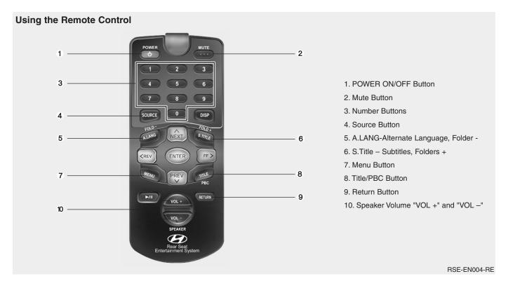
In addition to buttons and functions available from the RSE control panel, the remote control has several additional buttons and operation control functions. The remote control is an infrared device and should be pointed at the RSE monitor for best results.
