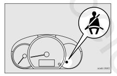
If the ignition switch is turned to the "ON" position or the operation mode is put in ON without the driver's seat belt being fastened, a warning light will come on and a tone will sound for approximately 6 seconds to remind you to fasten your seat belt.
