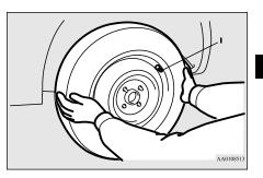
Install the wheel nuts with their tapered ends facing inward, then tighten by hand until the wheel is no longer loose.
