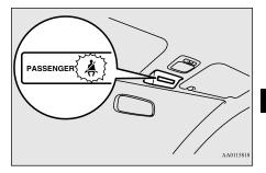
When the ignition switch is turned to the "ON" position or the operation mode is put in ON, this indicator normally comes on and goes off a few seconds later.
