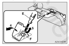
Push and pull the child restraint system in all directions to ensure it is firmly secured.
