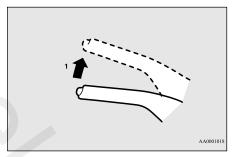
1- Pull the lever up without pushing the button at the end of hand grip.
