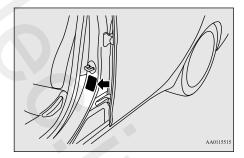
This placard shows the maximum number of occupants permitted to ride in your vehicle as well as "the combined weight of occupants and cargo" (A), which is called the vehicle capacity weight. This placard also tells you the size and recommended inflation pressure for the original equipment tires on your vehicle. For more information, refer to "Tires" on page 9-12.
