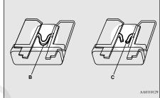
B- Fuse is OK C- Blown fuse
