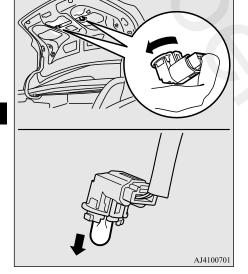
2. To install the bulb, perform the removal steps in reverse.
