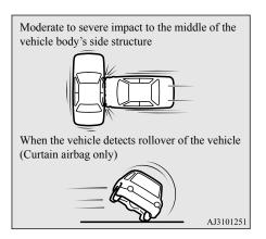
The seat belts in your vehicle are your primary means of protection in an accident. The SRS side airbags and curtain airbags are designed to provide additional protection. Therefore, for your safety and the safety of all occupants, be sure to always wear your seat belts properly.
