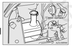
When freezing weather is anticipated, flush out the water in the reservoir by operating the pump. Fill the reservoir with windshield antifreeze (not radiator antifreeze), and operate the system for a few seconds to flush out the residual water.
