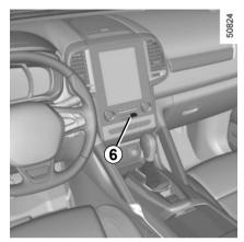
The switch **6** controls the doors and the boot simultaneously.
