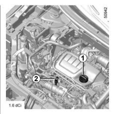
Do not exceed the **max** level and do not forget to refit cap **1** and dip-stick **2**.
