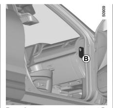
Fuses in passenger compartment B on the vehicle with stop and start function
