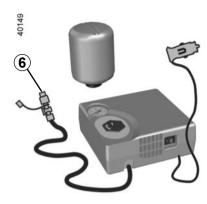
Once the tyre is correctly inflated, remove the kit: slowly unscrew the inflation adapter 6 to prevent any repair product from escaping and store the container in plastic packaging to prevent the product from escaping.
