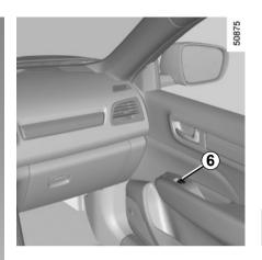
Avoid resting any objects against a half-open window: there is a risk that the electric window winder could be damaged.
