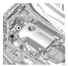
On the right-hand side of the vehicle, you will need to remove the filler neck **4** for the windscreen washer tank to access the bulbs. To do this:
