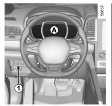
Instrument panel A: lights up when the driver's door is opened. When the ignition is switched on, turn wheel 1 to set the brightness of the instrument panel.
