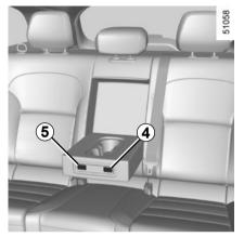
Depending on the vehicle, if you lower the rear seats armrest, there is a rear seats heating controller on the rear armrest.
