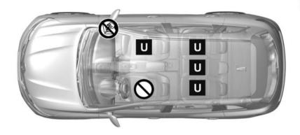
Check the status of the airbag before fitting a child seat or allowing a passenger to use the seat.
