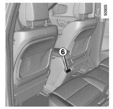
The sockets USB can also recharge accessories with a maximum power rating of 10.5 Watts (voltage: 5V) per socket, which have been approved by our Technical Department.
