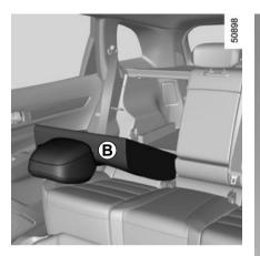
The configuration of the two-seat bench with the small seatback **B** pulled down, does not allow the central seat to be used as it would be impossible to buckle the seat belt (belt buckles inaccessible).
