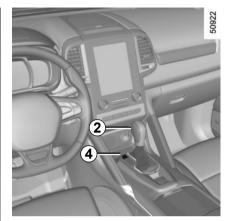
When setting off, if the lever is locked in position **P** even though you are pressing the brake pedal, the lever can be released manually. To do this, unclip the flap 4, then insert a tool (with a hard rod to it) into the hole and press the button 2 at the same time in order to unlock the lever.
