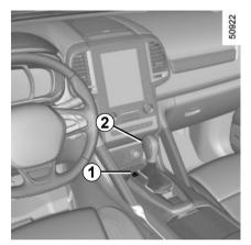
When setting off, if the lever is locked in position P even though you are pressing the brake pedal, the lever can be released manually. To do this, unclip the flap 1, then insert a tool (with a hard rod to it) into the hole and press the button 2 at the same time in order to unlock the lever.
