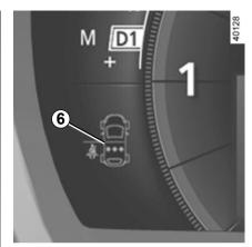
Check that the rear passengers are wearing seat belts and that the number of seat belts shown as fastened corresponds to the number of rear seat places occupied.
