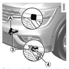
Only use the front towing point A and the rear towing point 5 (never use the driveshafts).
