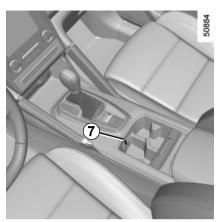
Raise the button 7 to ventilate the storage according to the temperature set by the air conditioner. Lower the button to stop the function.
