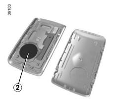
When refitting, proceed in the reverse order, then press one of the buttons on the card four times, close to the vehicle: the message will disappear.
