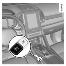
Switching on Press switch 5 on the side showing 5. Warning light to comes on, lit green, and the message "Adaptive cruise ctrl" appears on the instrument panel, accompanied by dashes to indicate that the cruise control function is activated and waiting to store a cruising speed.
