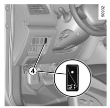
**Using the dashboard control**Depending on the vehicle, press and hold switch **4**.
