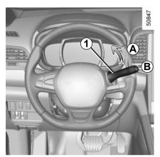
The blade on the driver's side must always be above the passenger-side blade. If this is not the case, a quick sweep of the windscreen wipers should be performed once the vehicle is travelling at over 4 mph (7 km/h).
