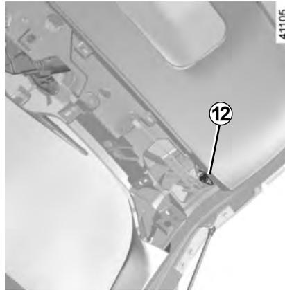
Turn bulb holder **12** fully anticlockwise and change the bulb.
