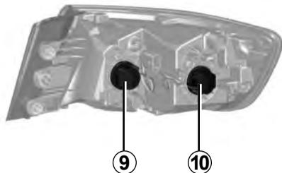
Refit the bulb holder and push the unit in fully until it locks in place.
