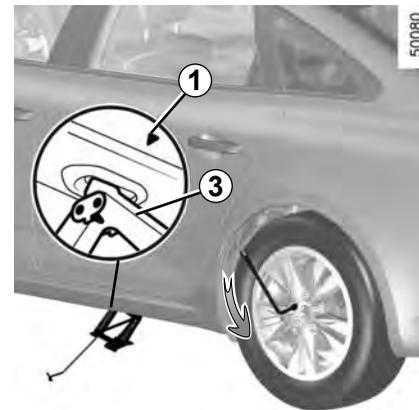
Crank up the jack by hand at first to align the base plate (which should be inclined further inwards than the jack head).
