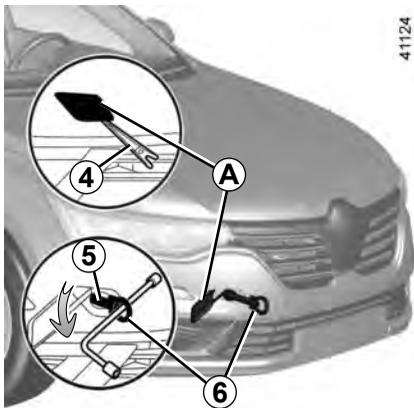
Only use the front 5 and rear 7 towing points (never use the driveshafts or any other part of the vehicle).
