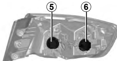
Refit the bulb holder and push the light unit in as far as it will go.
