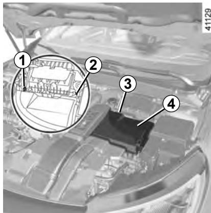
Lift the box cover **3** located behind the battery, then lift the battery half-cover **4**.
