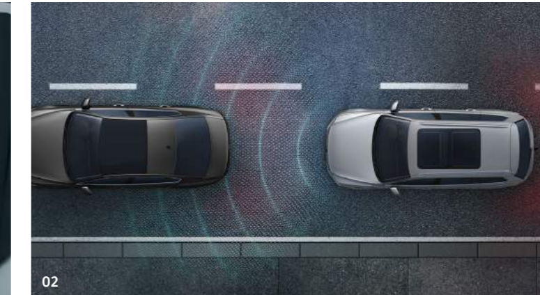
02 Adaptive Cruise Control (ACC), including Front Assist radar sensor controlled distance monitoring system, City emergency braking system, cruise control and speed limiter offers you intelligent control of your driving speed by automatically adjusting acceleration and braking. Whether around town or on the motorway, the system will adjust your speed to that of the vehicle in front, keep your specified distance, warn if you are approaching too fast and, in an emergency situation, generate enough braking force to try to reduce the severity of a collision or possibly even prevent the collision entirely. Image shown is for illustration purposes only and may not necessarily reflect UK specification.
