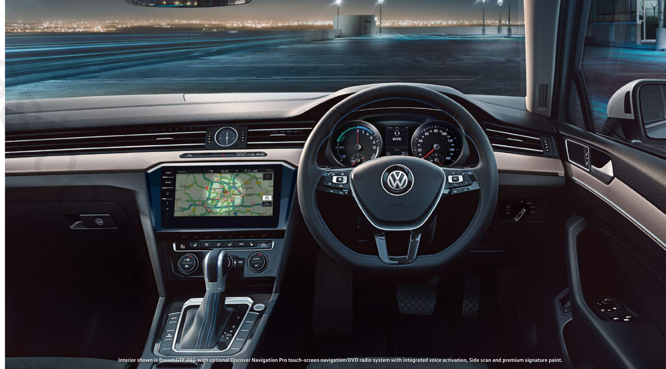
03 At the press of a button next to the gear lever, the driver can select e-mode. All-electric e-mode is ideal for urban driving, providing near silent, emission-free operation when driving in town or residential areas up to a distance of 31 miles 2 . The Passat GTE will automatically start in 'e-mode' for greater efficiency, but should the battery have insufficient charge, or in cases of extreme low temperature, the GTE's TSI petrol engine will cleverly take over.
