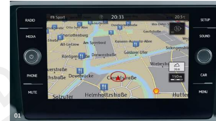
01 The Discover Navigation touch-screen navigation/radio system with Car-Net 'Guide and Inform' 1 offers Volkswagen Media Control 2 , allowing remote control of the infotainment system via a smartphone or tablet, preloaded European navigation data, 2D/3D map view, three calculated route choices (Fast, Short and Eco), dynamic navigation based on TMC+, branded points of interest and Speed Limit Display 3 . 3-year's Car-Net 'Guide and Inform' access makes it possible to integrate 'traffic information online' into route guidance and transfer public and personal points of interest to the navigation system. The service also includes information for fuel pricing, parking space availability, weather and news feeds.
