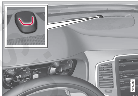
Lock and alarm indicator light on the dashboard
