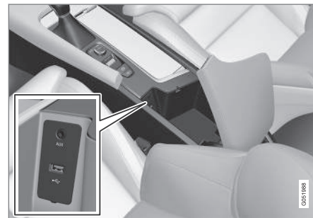
USB socket in the tunnel console
