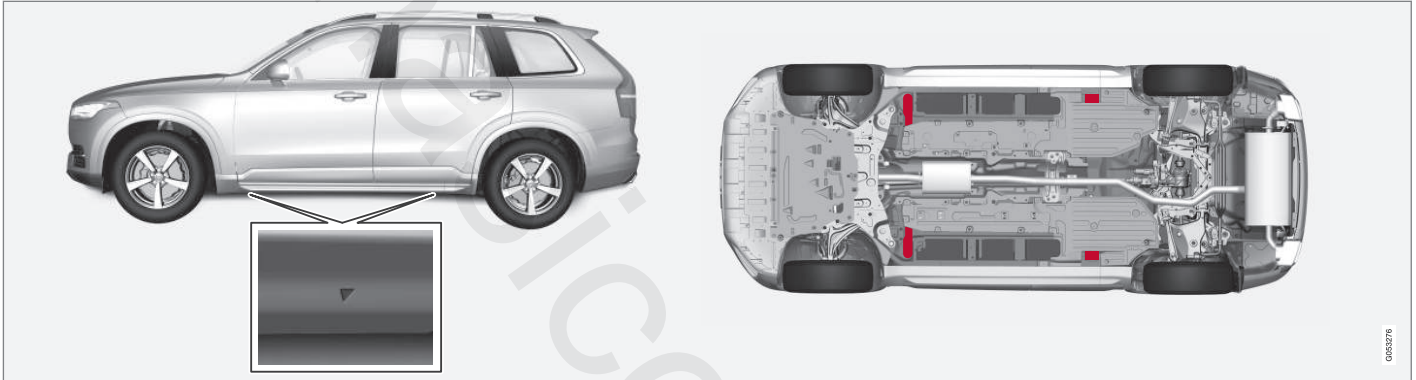
Location of the jack attachment points (triangles)/lifting points (red areas)
