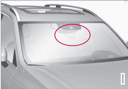
The marked area must not be obstructed in any way. This area of the windshield should always be kept clean
