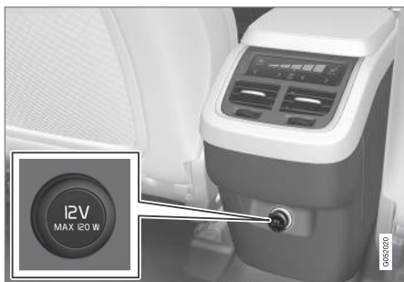
12-volt socket in the tunnel console for the second row of seats
