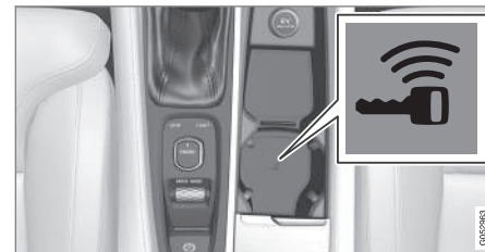
Backup key reader under the tunnel console cup holders
