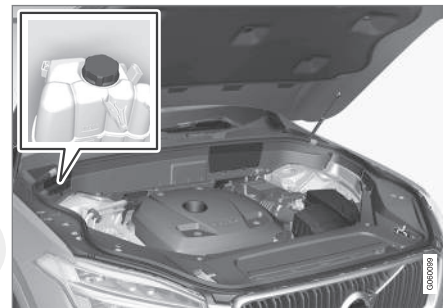
Coolant expansion tank
