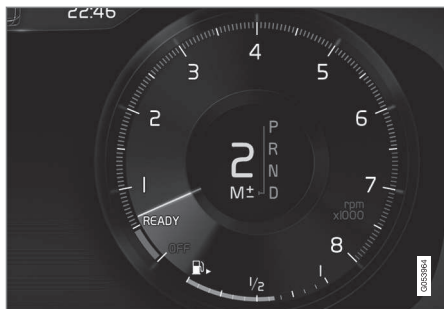
Manual shift indicator in the instrument panel 8 .
