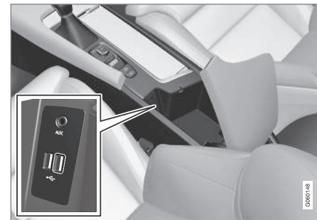
AUX/USB sockets in the tunnel console
