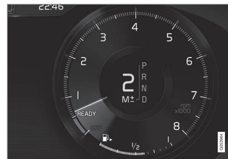
Instrument panel when the paddles are activated
