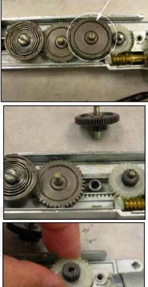
6. Remove the old plastic gear by pulling it straight up and out.
