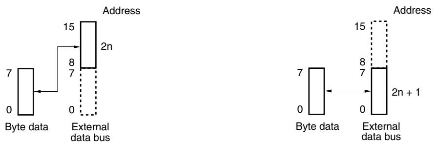
Figure 7-34 Left: Access to even address ( 2n ) Right: Access to odd address ( 2n + 1 )
